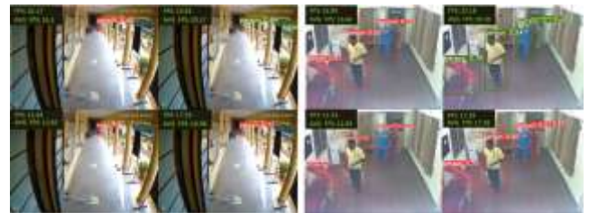
Figure 6: Detection of 'Person' class by YOLOv5, v6, v7 & v8.
